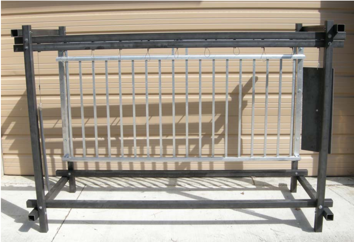
Figure 2: Section Mounted to Test Frame
