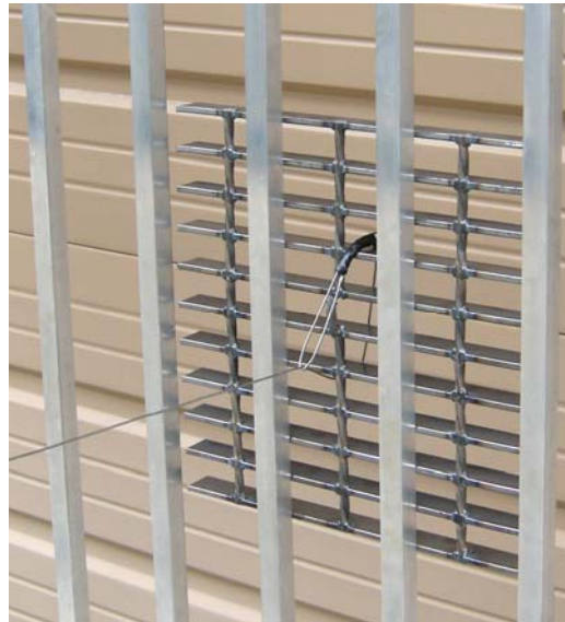
Figure 7: Uniform 50 lb/sqft load setup (typical)
