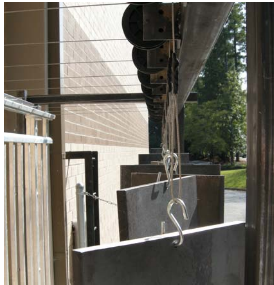
Figure 4: Loading Direction through Cables and Pulleys
